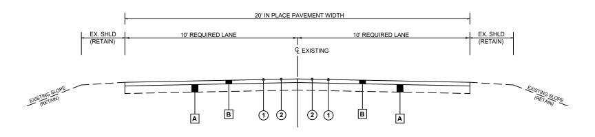
LEGEND NO. ITEM NO. **DESCRIPTION** "IN PLACE" EXISTING SUBGRADE / BASE (RETAIN) "IN PLACE" **EXISTING ASPHALT (RETAIN)** 433A-000 SCRUB SEAL "REQUIRED" "REQUIRED" 401B-106 MICRO-SURFACING SEAL COAT, TYPE II (APPROX. 25 LBS/SY)
